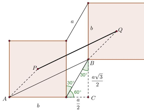
$$PQ^2 = AB^2 = AC^2 + CB^2 = \left(b + \frac{a}{2}\right)^2 + \left(\frac{a\sqrt{3}}{2}\right)^2 = b^2 + ab + a^2,$$
