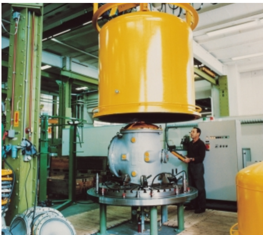
fig. 36 Leak testing of a GIS aluminium housing (ABB, Switzerland)
