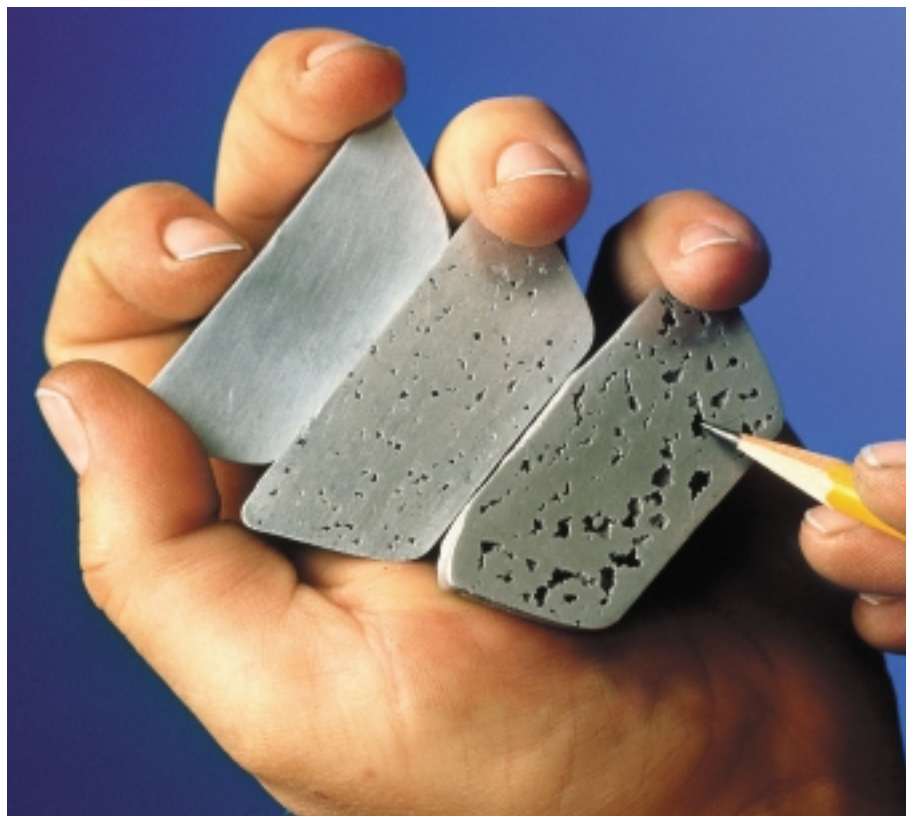
fig. 20 \text{SF}_6 -treated and untreated aluminum cast pieces in section
