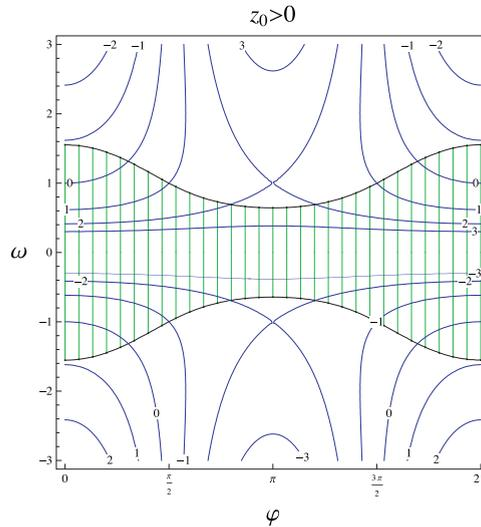
**Fig. 5.** Different curves for the gyrostatic moment onto the stability plane in  $(\varphi, \omega)$  for  $a = b = 1$  and  $z_0 > 0$ . The part of the curve inside the shaded region gives rise to a stable equilibrium point, whereas the equilibrium is unstable in the outer part.
