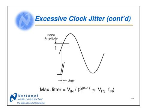
As the clock timing changes slightly, there is a change in the exact point of sampling. This causes the ADC to sample a higher or lower point in the signal than it should. The next point could have a different time variation, so a different change from the proper sampling point. The result is a lot of variation in the signal sampling point and degraded dynamic performance of the ADC.
