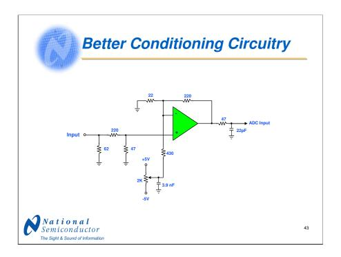
This is a much better solution, The amplifier is operated at a gain of about 11.5 (don't forget the effect of the 430-Ohm resistor on gain!) and the input is padded down so that the overall gain from input to output is about 2. The amplifier is happy with the high gain, but take care to watch gain bandwidth requirements.
