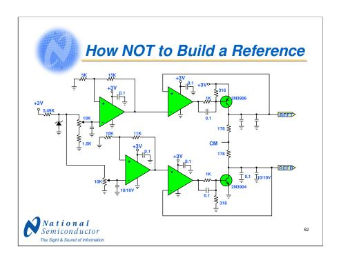
The problem here may not be obvious at first glance, but including the common-emitter gain of a transistor in the feedback loop of an amplifier is a recipe for high frequency oscillation. Also, this circuit has twice as many op-amps as needed and too many different resistor values, which manufacturing people <u>really</u> dislike!
