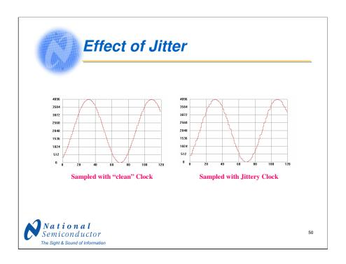
These plots from National's WaveVision software show the effects of excessive clock jitter. The noise on the signal is apparent.
