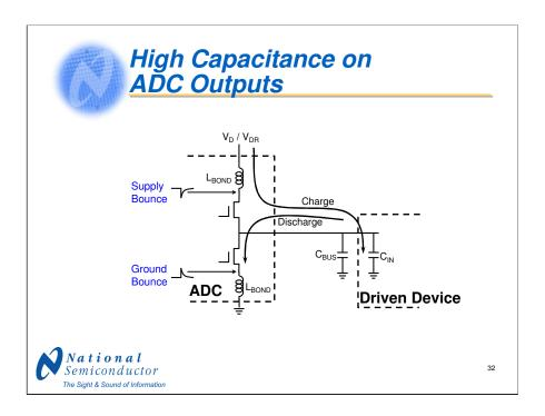
Charging bus and device input capacitances causes noise on the supply line, as we have discussed. Discharging these capacitances adds noise to the ADC substrate (die ground) and supply bus, which can appear at the input as noise. The task, then, is to minimize these currents.
