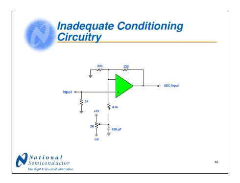
This simple circuit has a nominal gain of +2. The arm of the potentiometer is properly bypassed to prevent the gain from changing with a change of bias setting.
