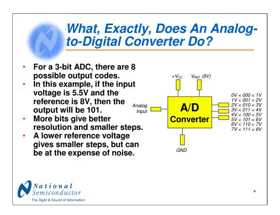
Here is an example of a 3-bit A/D converter. Because it has 3 bits, there are  $2^3 = 8$  possible output codes. The difference between each output code is  $V_{BEF} / 2^3$ .
