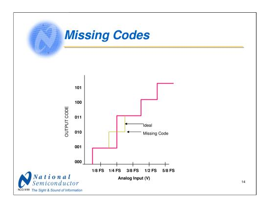
When no value of input voltage will produce a given output code, such that the code in question never appears in the output, that code is missing from the transfer function and is known as a <u>missing code</u>.
