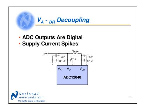
The digital output drivers of the ADC provide fairly fast edge rates (rise and fall times). This causes the output drivers to draw varying amounts of dynamic supply current with fast rise times to charge whatever capacitance is on the outputs when the output data must go from a logic low to a logic high. The noise thus introduced on the output driver supply can upset any analog circuitry if that supply is not decoupled from the ADC output drivers.
