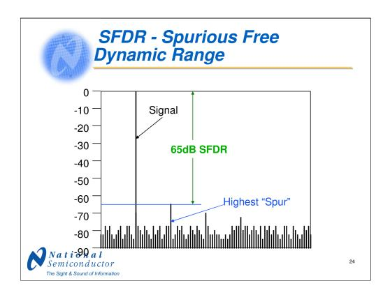
Spurious Free Dynamic Range (SFDR) is the difference between the value of the desired output signal and the value of the highest amplitude output frequency that is not present in the input, expressed in dB. Some ADC suppliers ignore harmonics when specifying SFDR, but this practice is valid only if those harmonics were present at the ADC input.
