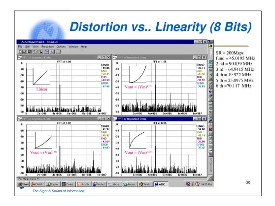
These FFT plots, made with our WaveVision software, shows the distortion that results with different amounts and types of non-linearity.
