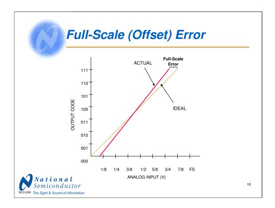
In an ideal A/D converter, the output code transition to full scale just barely occurs when the input voltage equals G \*  $V_{REF}$  \* (2<sup>n</sup> - 1.5) / 2<sup>n</sup>, where "G" is the gain of the converter (usually "1"),  $V_{REF}$  is the ADC reference voltage and "n" is the resolution (number of output bits) of the ADC.
