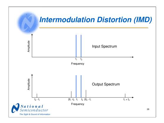
Any complex signal contains components at several frequencies simultaneously. Non-linearity in the converter's transfer function will not only cause distortion of a pure tone; it will also cause two or more signal frequencies to interact with each other to produce intermodulation products. When this happens, the result is called <u>Intermodulation Distortion</u>, IMD.
