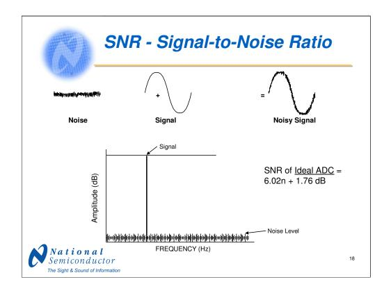
Signal-to-Noise Ratio (SNR) is the ratio of the output signal amplitude to the output noise level, not including harmonics or dc. A signal level of  $1V_{RMS}$  and a noise level of  $100\mu V_{RMS}$  yields an SNR of  $10^4$  or 80dB. The noise level is integrated over half the clock frequency.
