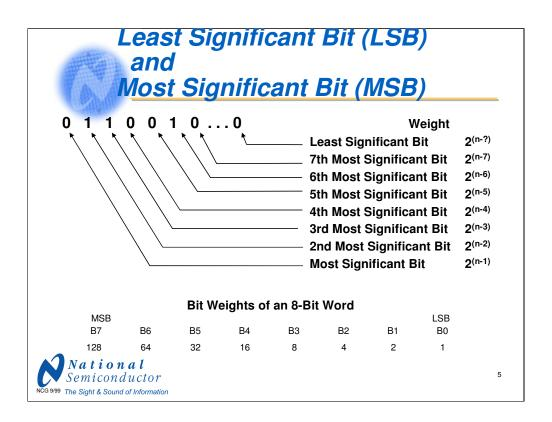
The Least and Most Significant Bits (LSB and MSB) are just what their name implies: those bits that have the least weight (LSB) and most weight (MSB) in a digital word. For an n-bit word, the MSB has a weight of  $2^{(n-1)} = 2^n / 2$  where "n" is the total number of bits in the word. The LSB has a weight of 1.
