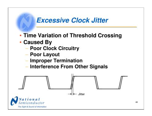
Jitter is the time variation of the threshold/zero crossing of a signal.
