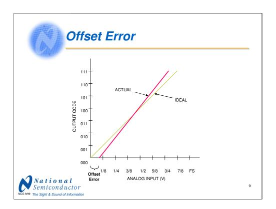
In an ideal A/D converter, an input voltage of q / 2 will just barely cause an output code transition from zero to a count of one. Any deviation from this is called Zero Scale Error, Zero Scale Offset Error, or Offset Error. This error is positive or negative when the first transition point is higher or lower than ideal, respectively. Offset error is a constant and can easily be factored or calibrated out. Offset error may be expressed in percent of full scale voltage, Volts or in LSB.
