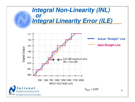
Integral Non-linearity, INL, (also called Integral Linearity Error or ILE and Linearity Error or LE) describes the departure from an ideal linear transfer curve for an ADC (or a DAC). INL does not include quantization errors, offset error, or gain error. It is a measure of the straightness of the transfer function and can be greater than the differential non-linearity. The size and distribution of the DNL errors will determine the integral linearity of the converter.
