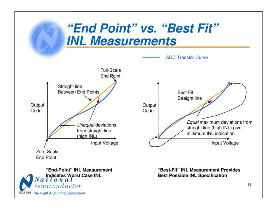
There are two methods of measuring Integral Non-Linearity (INL):
