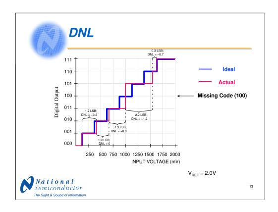
In an ideal converter, the code-to-code transition points are exactly 1 LSB apart. In an 8-bit ADC, for example, these changes are separated from each other by 1 LSB, or  $^{1}/_{256}$  of full-scale. The difference between the ideal 1 LSB and the worst case actual input voltage change between output code transitions is called Differential Non-Linearity.
