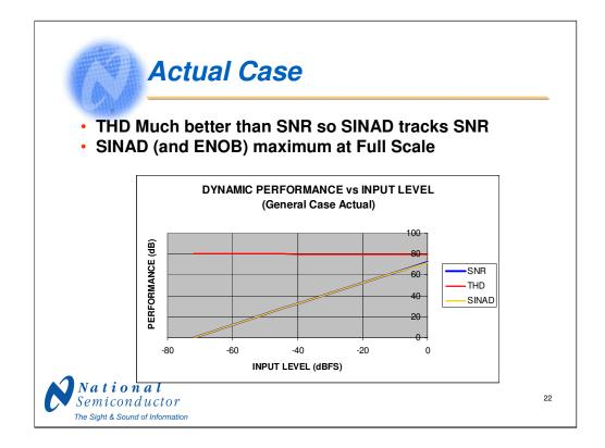
The THD performance of today's ADCs is so good that it does not change much (if any at all) with input level, so SINAD is dominated by SNR, which is not as good as THD, resulting in a SINAD that closely tracts SNR.
