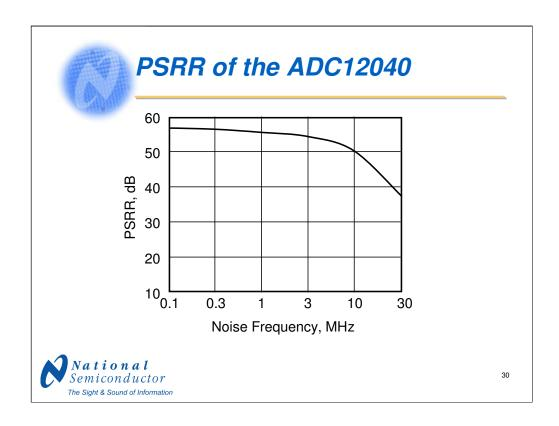
The PSRR of the ADC12040 is excellent, yet PSRR does degrade with higher frequencies. To degrade just 8dB from 100kHz to 10MHz, however, is exceptionally good for any ADC.
