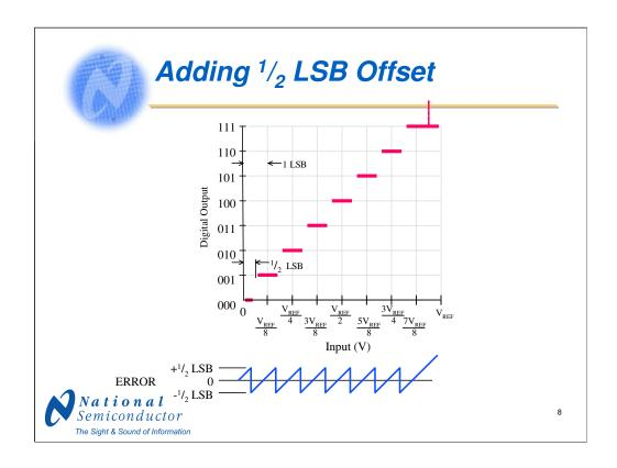
If we add  $^{1}/_{2}$  LSB offset to the ADC input, the output code will change  $^{1}/_{2}$  LSB before it otherwise would. The output changes from 000 to 001 with an input value of  $^{1}/_{2}$  LSB rather than 1 LSB and all subsequent codes change at a point  $^{1}/_{2}$  LSB below where they would have changed without the added offset.
