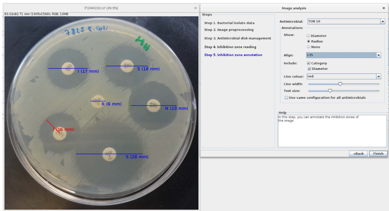
Fig. 1. Screenshot of AntibioGramJ. On the left, the image of a plate is shown with the diameter and category (Intermediate, Susceptible, Resistant, Not Available) associated with each antimicrobial disk.
