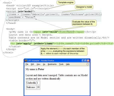
Fig. 3. JST2 example and its visualization on an internet browser
